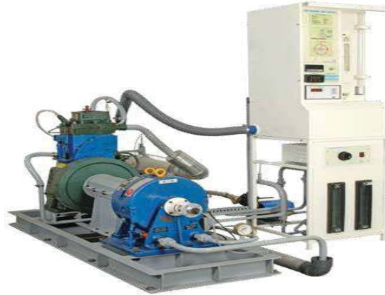
FIGURE 4. VCR Engine Setup
